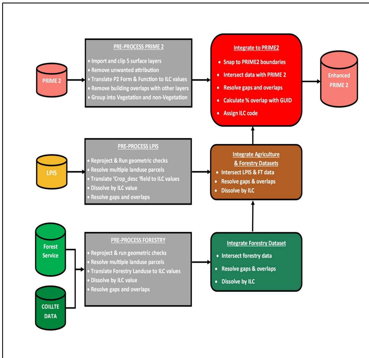
Figure 4.1: Pre-processing core vector data integration workflow
